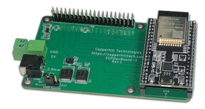
Copperhill Technologies, a provider of embedded systems for CAN Bus development, introduces the espBerry, a new line of ESP32 development boards. The espBerry series includes the basic espBerry board, a dual CAN-Bus channel system, and an NMEA 2000 & NMEA 0183 development board. Further configurations are in the works. Still, the espBerry concept supports engineers with the implementation of additional HATs. Open-source code samples support all hardware configurations.
