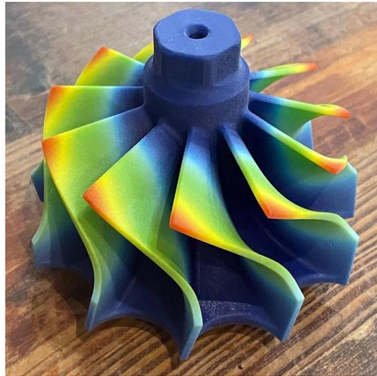
*Custom Plugin Allows Users to Create 3D Printed Full-Color Models with Results Contours*
