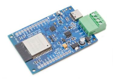
The ESP32-CANBus modules by Copperhill Technologies, with their integration of WiFi, Bluetooth, and Bluetooth LE, allow a wide range of employment, including industrial, automotive, maritime, and Internet of Things (IoT) applications. The ESP32 series of modules support an extended operating temperature range of -40°C to 85°C and are suitable for commercial application development.
