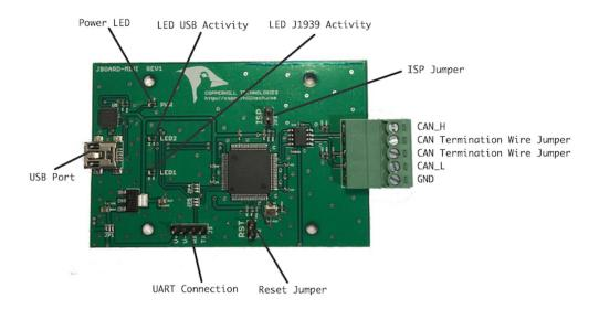
Copperhill Technologies offers a variety of hardware modules equipped with an On-Chip SAE J1939 Protocol Stack, relieving the end user from implementing third-party source code and avoiding license fees. The programming of J1939 network communication is accomplished through accessing a standard serial port, making the development virtually independent of the operating system.
