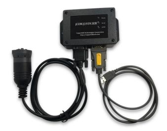
The JCOM.J1939.SER gateway is a high-performance, low-latency, serial vehicle network adapter for SAE J1939 applications. It allows any host device with an RS232 or USB port to monitor SAE J1939 data traffic and communicate with the SAE J1939 vehicle network.
