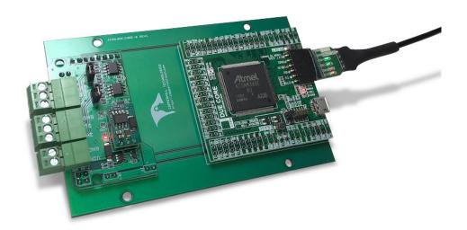
Copperhill Technologies announced the release of its JCOM.DUE.CORE gateway, a programmable embedded system based on the Arduino Due, supporting two USB and two CAN Bus ports.
