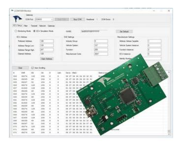
Copperhill Technologies introduces its jCOM.J1939.USB gateway, a vehicle network adapter to monitor, simulate, and record SAE J1939 data traffic.
